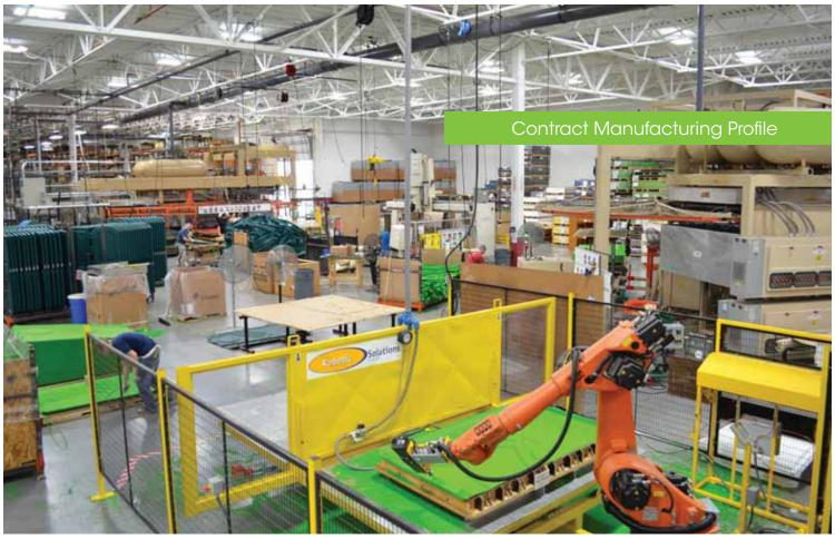
Inside Hampel's 160,000 ft², ISO 9001:2008-certified plant, there are 10 workcenters, each supported by the latest in forming equipment as well as five and six-axis robotic post-molding CNC trim cells. Hampel uses CMMs and supporting inspection software for quality assurance.
